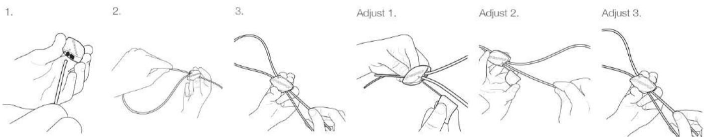
Ensure a minimum 75 mm of tail wire exits the hanger.
